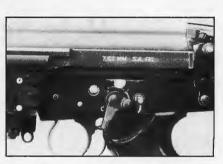
Israeli FAL lower receiver: Hebraic selector markings have been milled off and replaced with 'S' and 'F' on the semiautomatic version. Long legs on the selector prevent its movement to the full-auto position. Note ringed magazine catch release and takedown lever which remains in the early location in back of the upper receiver.
